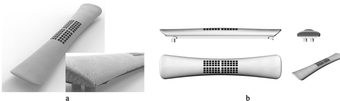
Figure 6: Design scheme of solar panel cleaning robot convenient to transportation.
