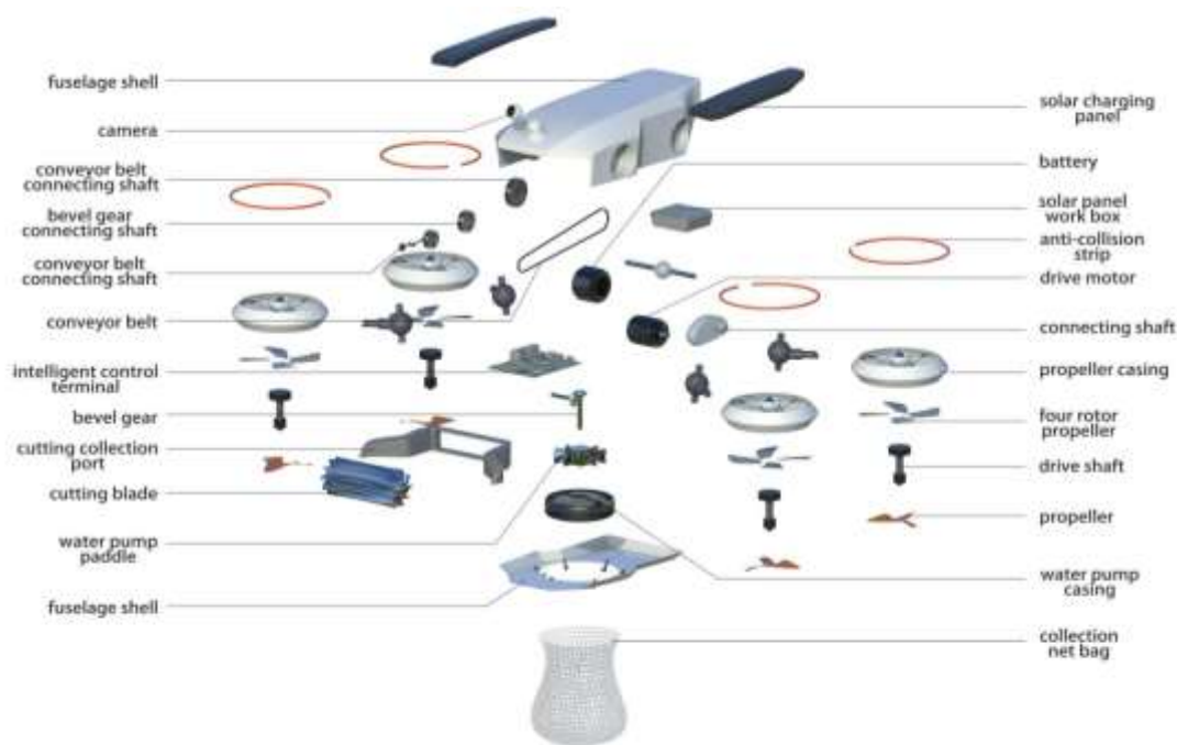
Figure 8: Explosion diagram of product structure.
